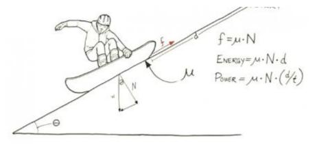
Friction will occur at any place where two surfaces come into contact with each other. Friction can cause energy losses that create unwanted heat, deformation, and wear. This can reduce the lifetime and increase the cost of the products you design.
